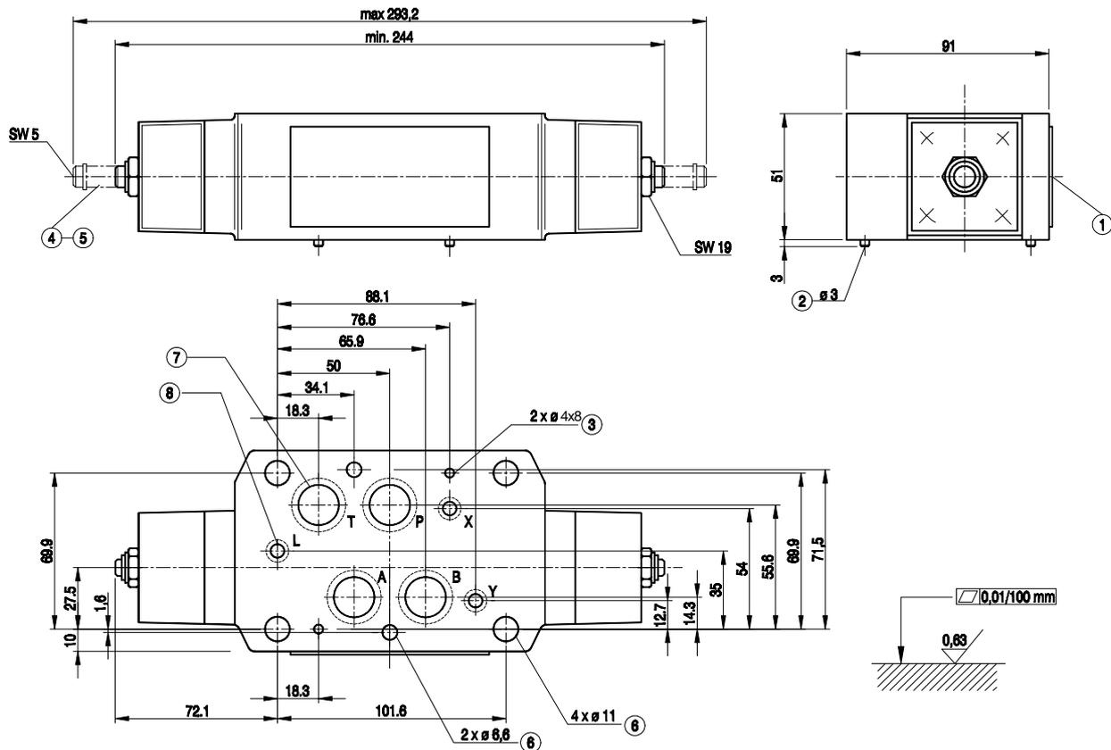
Admissible surface roughness and flatness deviation for a subplate face.
