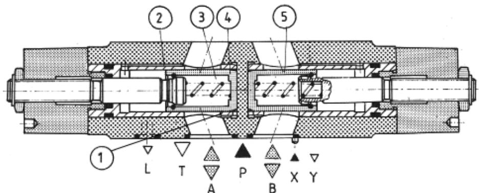
Hydraulic fluid in line A flows to a user through the throttle position 1. At the same time, the fluid being under operating pressure reaches the spring loaded side 3 of the spool 4 via the line 2. The spool 4 is thus hold in the throttle position by both spring and pressure force.
