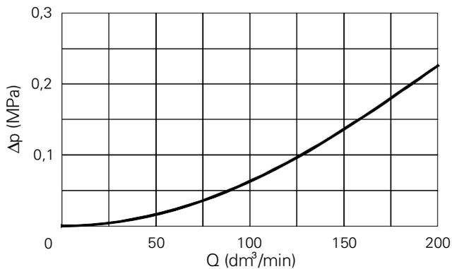
Pressure drop  $\Delta p$  in relation to flow rate  $Q$  with constant throttling
