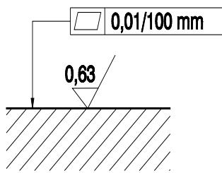
Admissible surface roughness and flatness deviation for a subplate.
