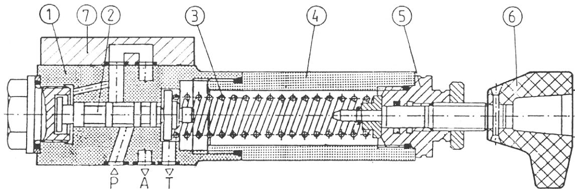
The spool 2 is held in neutral position in the housing 1 by the spring 3. At the same time pressure in line A affects the spool surface opposite the spring. The valve is open in initial position. The spring force is set by turning the hand knob 6 of the setting element 5, which is screwed in the sleeve 4. If pressure exceeds the value set at the spring, the spool moves along and reduces the flow from P to A.
