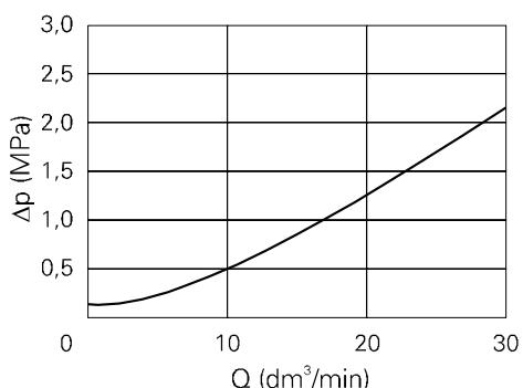
$\Delta p = f(Q)$  - pressure drop at check valve in relation to flow rate
