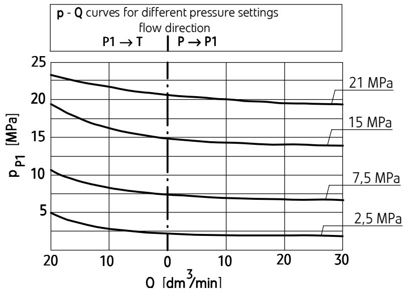
Characteristic curves of minimum pressure drop in relation to flow rate in the direction of flow  $P - P1$
