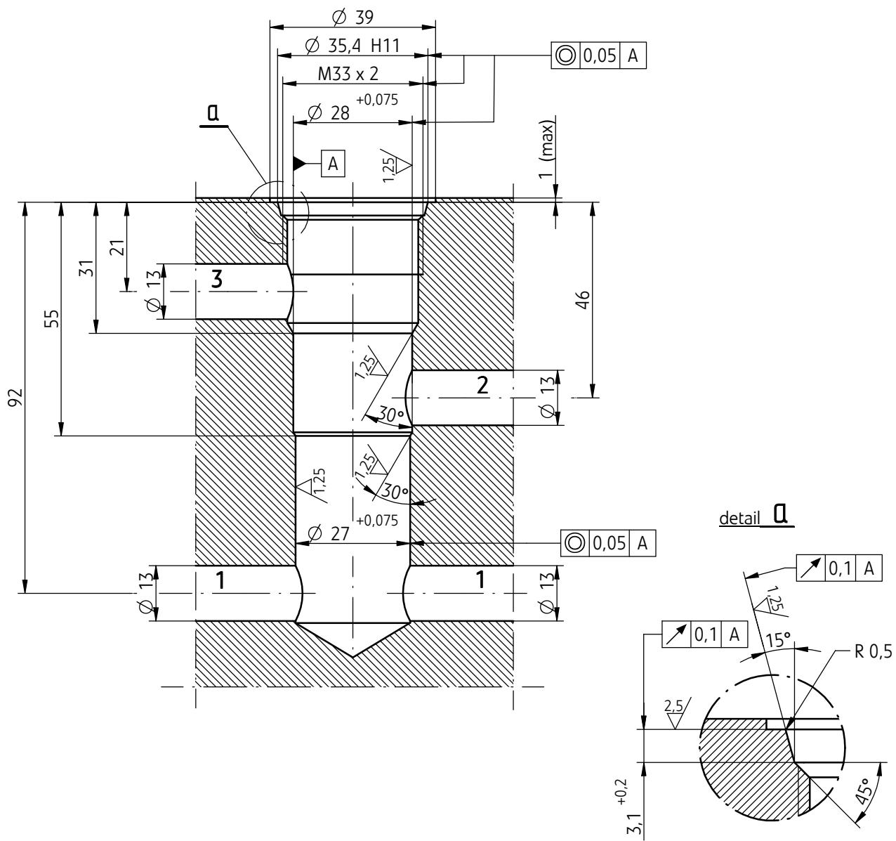
Connection of pipelines G3/4 (G4)
