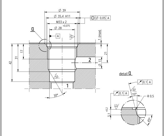
Connection of pipelines G3/4 (G4)
